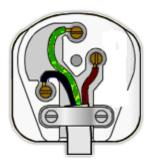
Here, the red and the black wires are called the supply wires, while the green wire is for safety.
